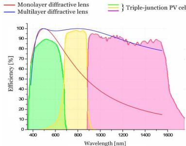
Fig. 7: 1st order diffraction efficiency compared with a triple junction PV cell
