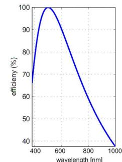
Fig. 2: diffraction efficiency for PMMA
