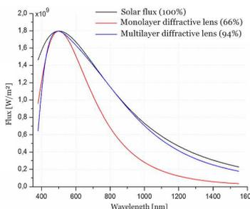
Fig. 6: flux at first order compared with solar flux
